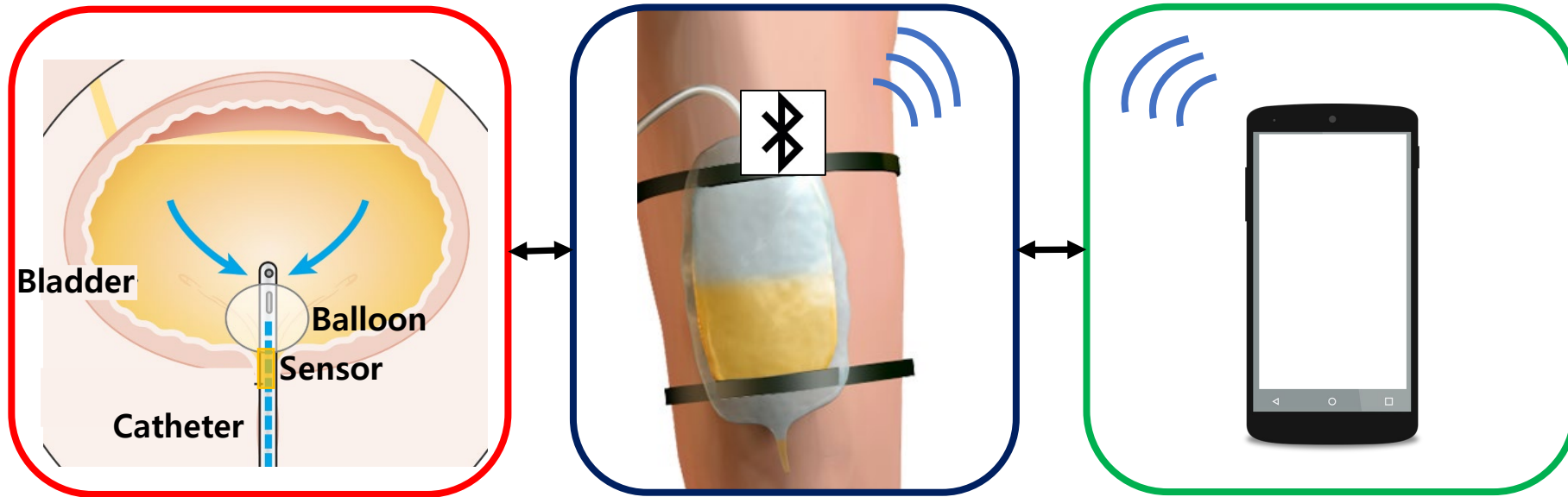
Wireless readout and control approach showing sensor embedded (inserted urinary catheter) on a cylindrical surface
